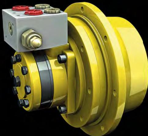
Wheel drives come in 5 sizes with a maximum torque ranging between 800 and 3,500 Nm. These models are suitable for track drive and wheel drive applications due to the relatively high load supported by the bearings (8,000 kg in the EH models). Several accessories are available (including static brake, disengagement system, and control valves).
